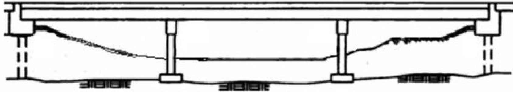
Integral continuous superstructure
